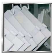
พ่นด้วยสีคุณภาพ 2 Tone Hammer Completely finishing with acrylic urethane hammer-tone paint
